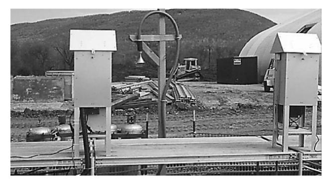
Figure 5-9. Example of properly placed extractive perimeter VOC inlet probe collocated with RMM time-integrated monitoring systems
