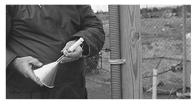
Figure 5-4. Example of sintered stainless steel inlet filter as part of a perimeter VOC FFMS
