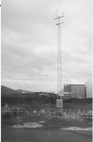
Figure 6-1. Example of a 10-meter meteorological station at a HTRW site
