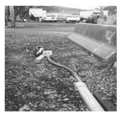
Figure 5-3. Example of heat-trace line layed above ground as part of perimeter volatile organic sampling system
